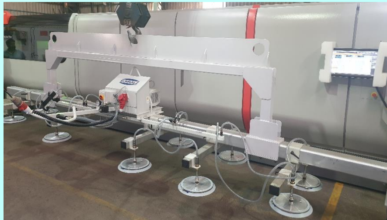
2 Ton, 6 meter Schmalz vacuum Lifter
